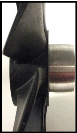
Flat Belt Cooling Fan (Old Style)
